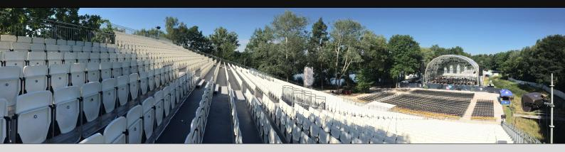
Seating options on these structures ranges from very simple bleachers (benches) which are compact to transport / store and are easy to install but are not very comfortable, though to 'tip up' seating. Conversely 'tip ups' are comfortable but are traditionally bulky requiring special steel cages or 'stillages' in which to transport and store them, they are also awkward to handle and inefficient to install.
