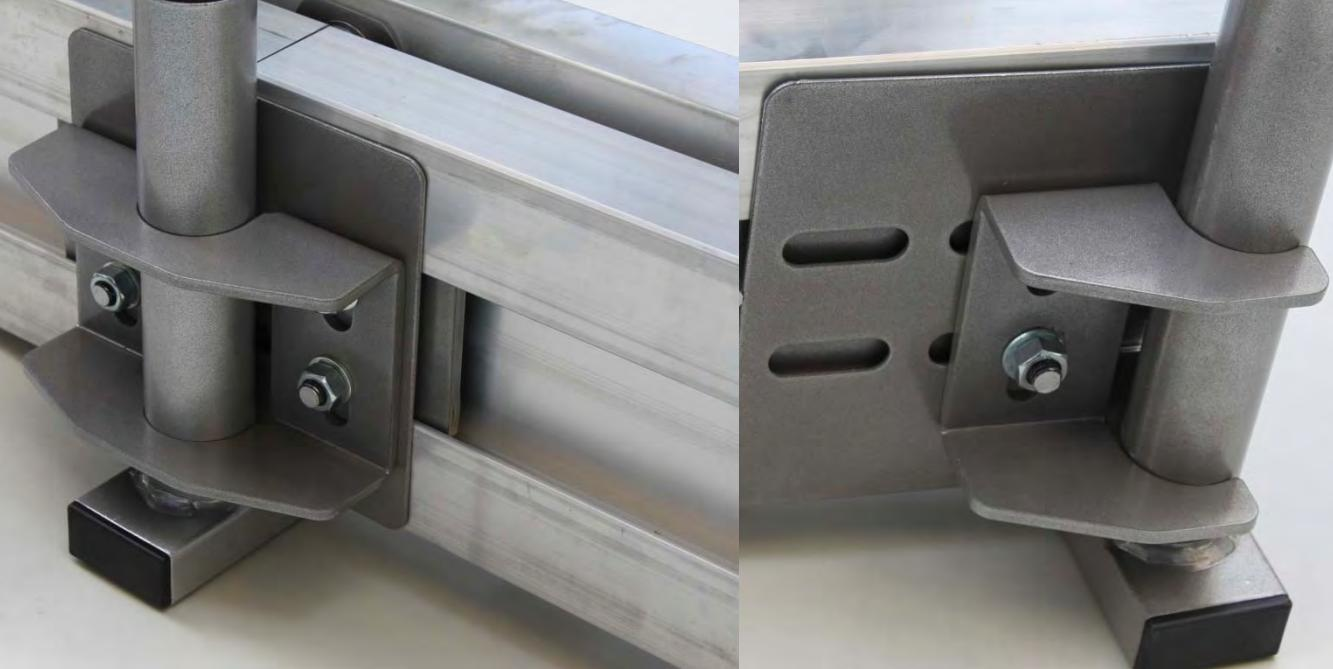
**nomad** seats can be applied to any temporary structure – scaffold systems – frame systems – SPS – our attachment system consists of extruded aluminium profiles to accommodate a 2.5M system span. Steel attachment clamps slide into the extruded profile and can be positioned anywhere so that any system span can be accommodated. Connector assembly's are also available so that profiles can be joined end to end.
