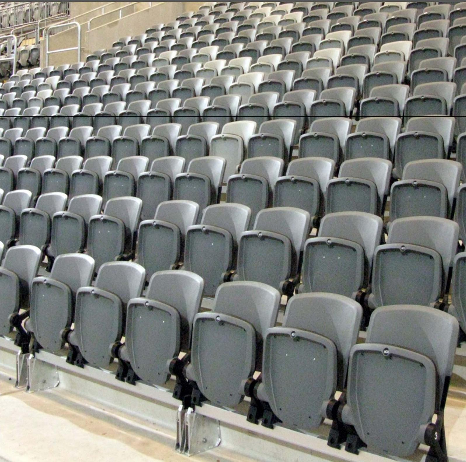
**fast – latch** mechanisms are arranged - predominantly in 3 seat modules – a small number of 2 seat modules are sometimes required to ensure that the maximum number of chairs will fit into the layout .
